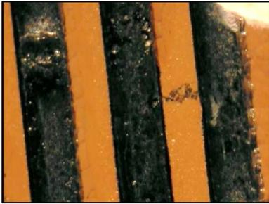
**Figure 9.** Dendrites Growth on Paste B boards under Customized #3 ECM Test
